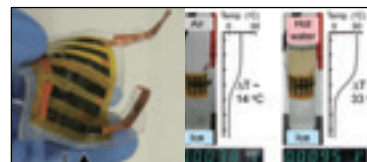
Fig.2 Flexible thermoelectric sheet based on p-type and n-type carbon nanotubes
