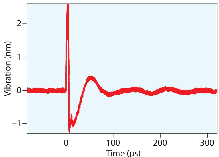
An atomic force microscope (AFM) probe is positioned atop a plant root (left) immersed in water. An extremely short laser pulse targeted some distance away creates a shockwave by heating and vaporizing water. The resulting vibrations in the plant root can be measured from the movement of the AFM probe (right).
