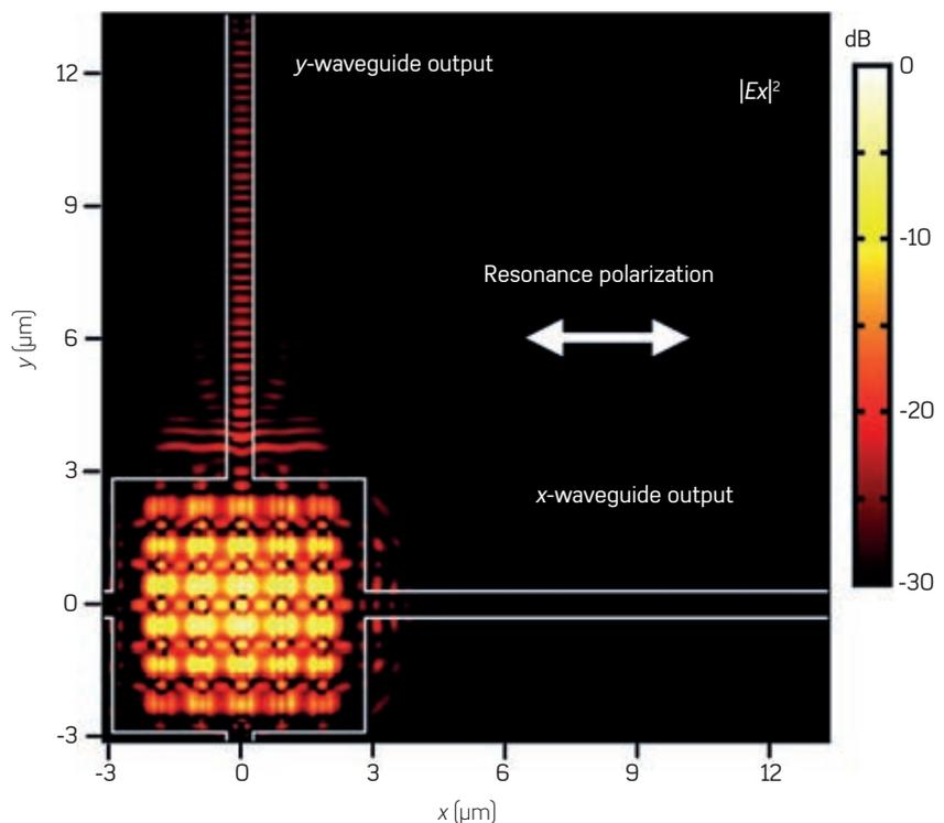
Simulation showing light exiting the VCSEL via the y waveguide only. By changing the lasing polarization, the output light switches to the x waveguide.
