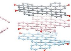
A star-shaped, triple-layered complex of flat carbon sheets can store surprising amounts of electronic charge.
