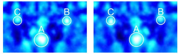
The DIANA device that Professor Daimon and his colleagues developed allows researchers to visualize the positions of atoms within material, such as the three atoms circled in these images. In a viewer, pairs of stereoscopic holograms combine to form a three-dimensional image.
