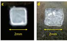
Mixing solutions of the PEG-PLLA and PEG-PDLA polymers forms a gel that is held together by stereocomplex formation.
