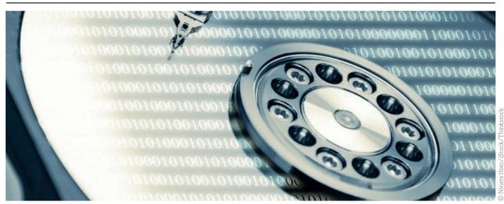
Layers of magnetic and non-magnetic materials are used in the read heads of computer hard drives.
