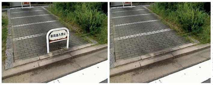
Diminished reality in action: Left panel is the original image, right panel is the resulting image with signpost removed via the new diminished reality process.
