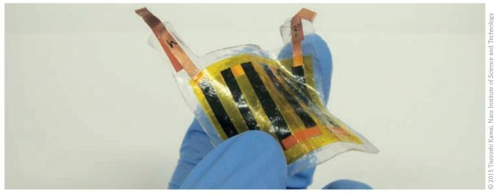
A bendable thermoelectric device made from modified carbon nanotubes can generate electricity from a temperature gradient.
