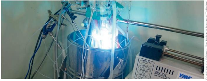
The photoreactor used to produce cyclobutanes.
