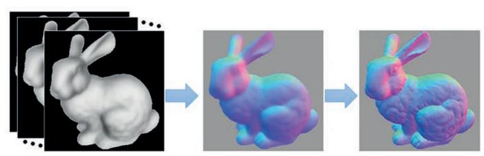
A new technology makes it possible to turn multiple pictures of translucent objects (left panel) into sharp and realistic 3D images.
