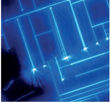
NAIST researchers hope to soon fabricate light-emitting diodes based on BP1T-CN, an n-type TPCO organic semiconductor crystal, which emits bright blue light when illuminated with ultraviolet radiation.
