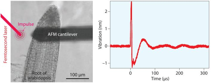
An atomic force microscope (AFM) probe is positioned atop a plant root (left) immersed in water. An extremely short laser pulse targeted some distance away creates a shockwave by heating and vaporizing water. The resulting vibrations in the plant root can be measured from the movement of the AFM probe (right).
