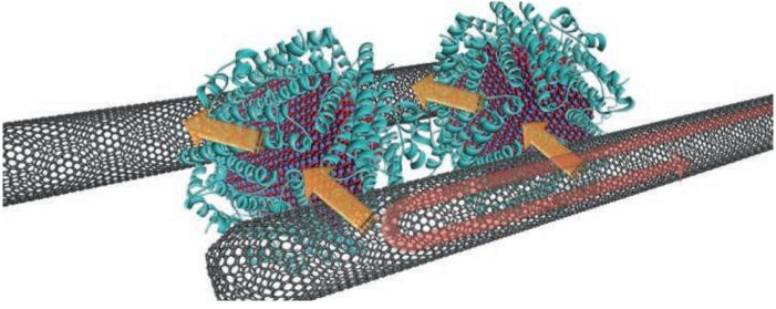
Carbon nanotubes (CNTs) linked by protein molecules (blue) with a semiconducting core (purple). Orange arrows show electric current flow from hot to cold CNTs. Red arrow indicates phonon scattering.
