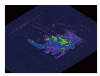
Visualization of information leakage paths based on large-scale EM field simulation techniques.
