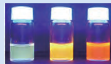
Luminescence from impurity-doped semiconductor nanoparticles
