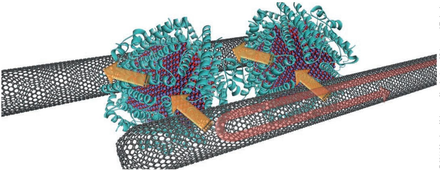
Carbon nanotubes (CNTs) linked by protein molecules (blue) with a semiconducting core (purple). Orange arrows show electric current flow from hot to cold CNTs. Red arrow indicates phonon scattering.
