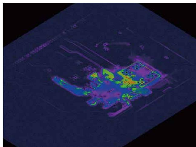
Visualization of information leakage paths based on large-scale EM field simulation techniques.
