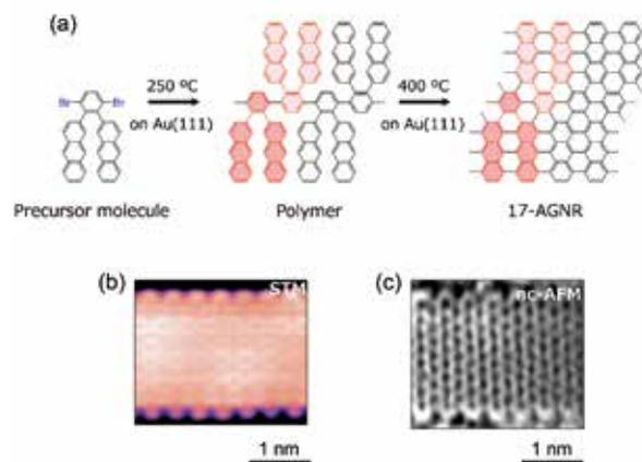
(a) Bottom-up synthesis scheme of 17-AGNR on Au(111), (b) high-resolution STM image, and (c) nc-AFM image of 17-AGNR.
