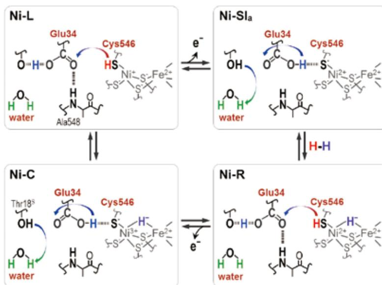
Protons are transferred between the NiFe active site and protein surrounding through the Cys546 and Glu34 residues during the catalytic reaction of [NiFe] hydrogenase.
