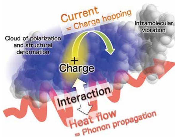
**Schematic illustration explaining the mechanism of the Giant Seebeck effect in organic semiconductors which is discovered in the NAIST Organic Electronics Laboratory.**
