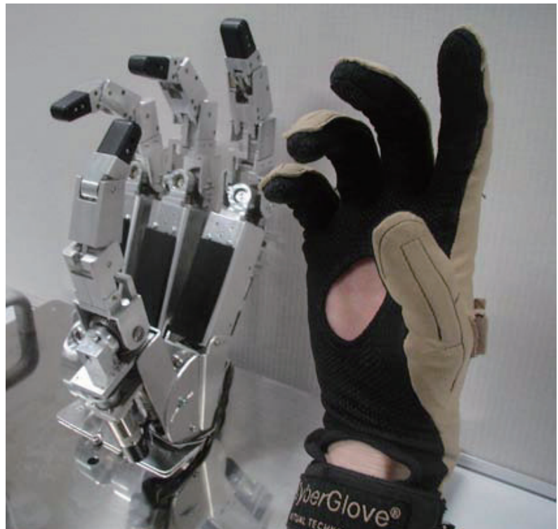
Motion transfer to the NAIST Hand (Ueda et al. , 2005, ICRA ).
